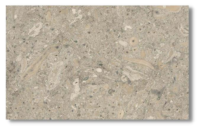
This light grey material, characterized by the presence of macrofossils, has long been a favorite limestone of architects, including Palladio. Recently rediscovered by modern architecture, it is suitable for both internal and external claddings, floors and interior staircases, as well as several other building components.
